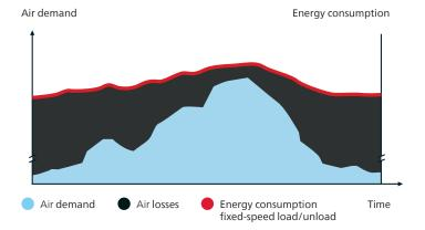
In almost every production environment, air demand fluctuates depending on different factors such as the time of the day, week or even month. Extensive measurements and studies of compressed air demand profiles show that many compressors have substantial variations in air demand.
